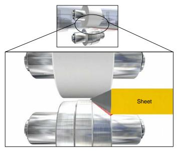
**Operation**: The embossing roller (bottom) displaces the burr (red) and chamfers the sheet edge (gray).
