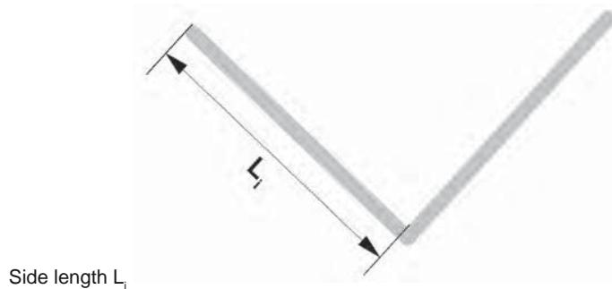
The following values for  $L_i$  were established in test sequences. The table does not take spring-back angle into account. This way the values for  $L_i$  are independent of materials:
