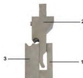
1 ... Torque stay rod with slide rail
