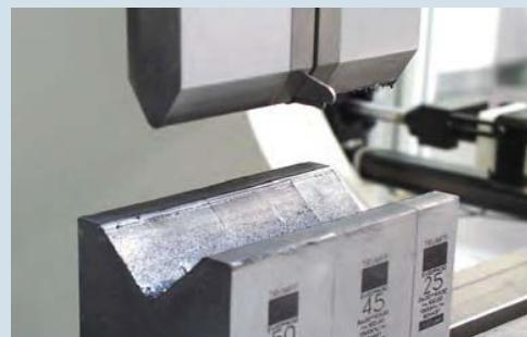
Early and regular maintenance servicing of the elements described above with an oil-soaked rag increases the service life and has a positive effect on the exactness of the bent parts. Determination of the cleaning interval here is always the responsibility of the machine operator.
