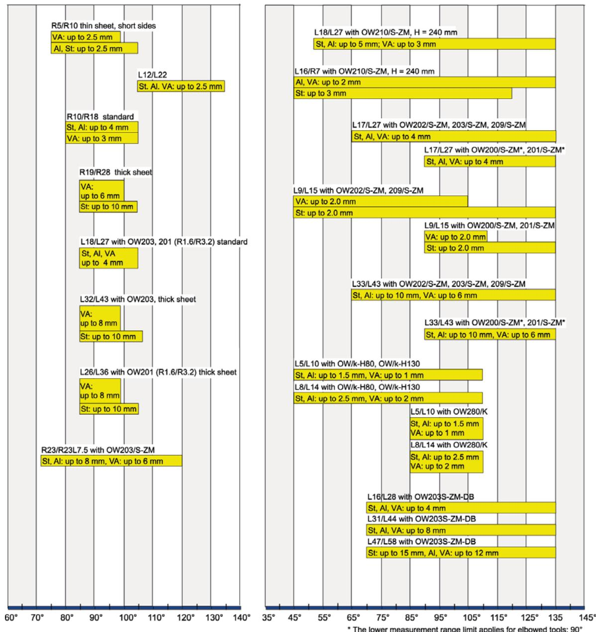
The angle range for the sensor disk combination R5/R10 (75° - 105°) does not apply for the tools OW200/K and OW201/K nor for OW200/S and OW201/S (86° tools).
