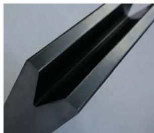
Coated Laserdur ZN dies are especially suited to processing galvanized sheets.
