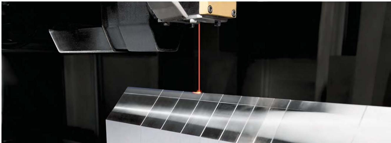
TRUMPF tools are laser-hardened. Thanks to utilization of a TRUMPF TLF high-performance laser with innovative special hardening optics, improvements over earlier laser hardening in terms of hardening depth and the width of the hardened zone have been achieved:
