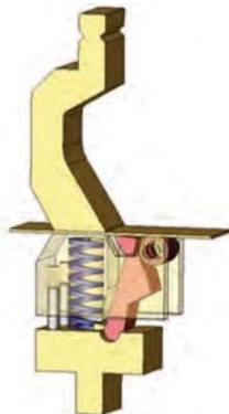
The swivel lever bends the link plate upwards
